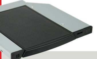
The DataPort DP27 removable drive is designed to fit into slimline optical disk drive bays, one of the most commonly found drive bays in computers today. That means that the DP27 can be installed into workstations, desktops, laptops, all-in-ones, government technology, or any other type of device. The DP27 ingests 2.5" hard drives or SSDs with the speedy 6G SATA interface.
